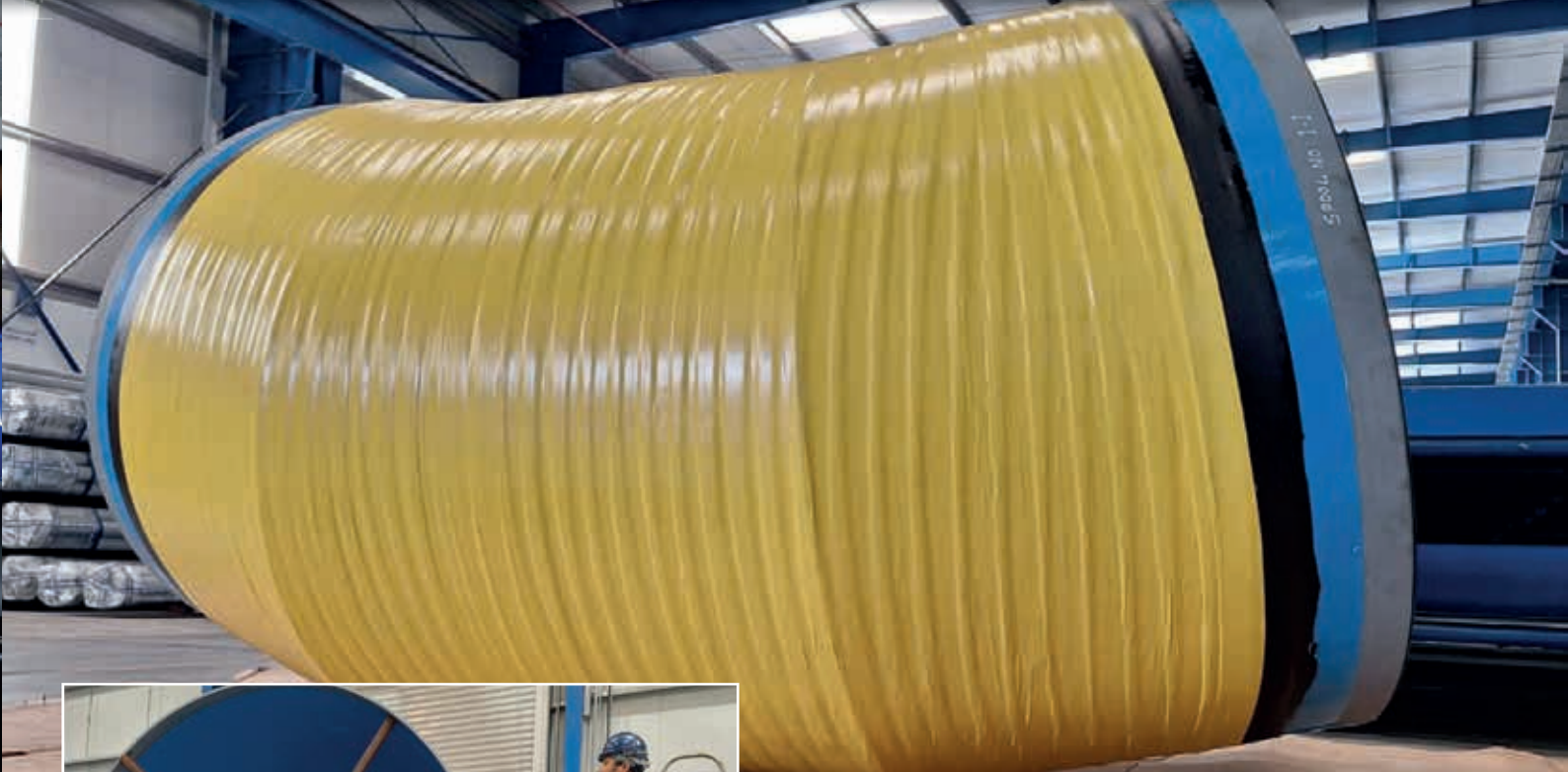
Above: A good example of a 50% overlapped tape wrap of Denso PVC SA 200 Tape, giving a double layer of outerwrap protection.
